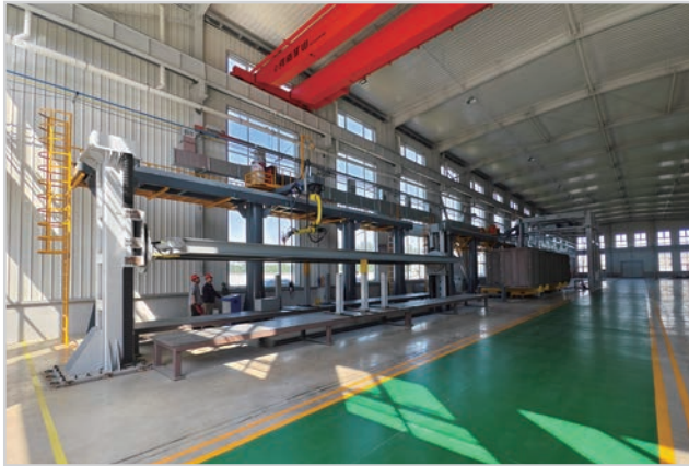
Robot Welding Production Lines for Solids Control Equipment
